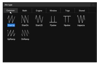
The oscilloscope can control the built-in waveform generator to output waveform with up to 50 MHz frequency and  $\pm 3$  V amplitude. Six basic waveforms plus multiple types of arbitrary waveforms are built-in
