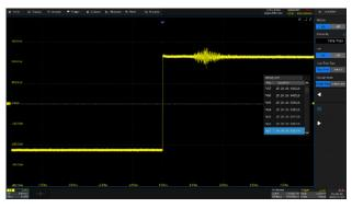
History function can record up to 124,000 frames of waveforms. The recording is executed automatically so that the customer can playback the history waveforms at any time to observe unusual events and quickly locate the area of interest using the cursors or measurements. The failed frames of the Mask Test can be stored as history
