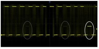
With a waveform update rate of up to 1,000,000 wfm/s, the oscilloscope can easily capture unusual or low-probability events. In Sequence mode, the waveform capture rate can reach 1,100,000 wfm/s
