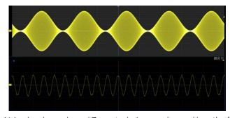
Using hardware-based Zoom technique and record length of up to 2 Gpts, users can select a slower timebase without compromising the sample rate, and then quickly zoom in to focus on the area of interest
