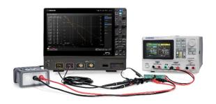
The oscilloscope can control the Built-in waveform generator, SIGLENT isolated USB AWG module or a standalone SIGLENT SDG generator, to scan the amplitude and phase-frequency response of the DUT, and display the data as a Bode Plot. This makes it possible to replace expensive network analyzers in some applications
