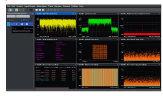
In the Spectrum Analyzer mode, it supports the functions of a Real-Time Spectrum Analyzer (RTSA) and Digital Down Conversion (DDC). The built-in signal analysis software SigVSA enables direct signal analysis of the output data of the DDC. The supported signal types range from simple Binary Phase Shift Keying (BPSK) to complex broadband signals, such as 4G LTE, 5G NR, IEEE802.11b/a/g/n/ac/ax/be and 4096QAM, and it also has rich measurement functions.
